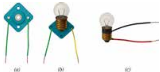
Figure : (a) An electric lamp holder with wires attached, (b) An incandescent lamp inside the lamp holder, (c) Wires connected to incandescent torch lamp with electrical tape
