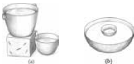
Figure : A water clock (a) Water flowing out-type, (b) Floating bowl-type
