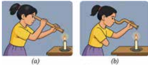
Figure : Viewing candle flame through (a) a straight pipe, (b) a bent pipe
