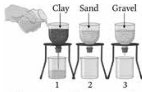
Figure : An activity to compare the flow of water through clay, sand and gravel
