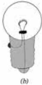
Figure : (a) A small incandescent lamp used in a torch (b) its simplified drawing showing the connection of wires to the terminals
