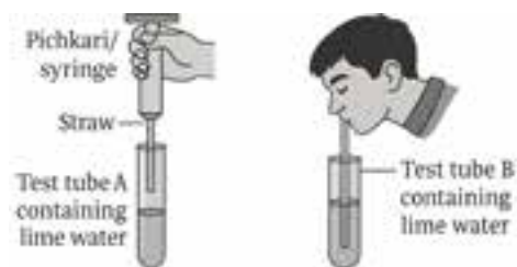
(a) Air is passed to lime water (b) Air exhaled into lime water
