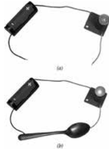
Figure : (a) Conduction tester, (b) Using the conduction tester for testing a material
