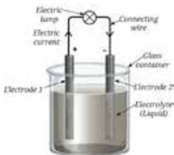
Simple representation of a Voltaic cell
