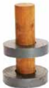
Force between two ring magnets
